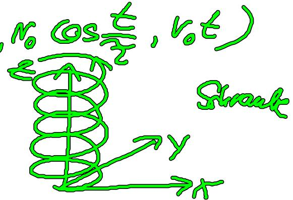
$$\Rightarrow \underline{r}(t) = \left( \frac{v_0}{\tau} \cos \frac{t}{\tau}, -\frac{v_0}{\tau} \sin \frac{t}{\tau}, v_0 t \right)$$
