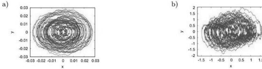
Fig. 1 - Simulated phase portraits of noise-induced oscillations of the Van der Pol system for \epsilon = -0.01 , \omega_0 = 1 , \tau = 0 , K = 0 : a) D = 0.003 ; b) D = 0.5 . Integration time: 300 time units.
