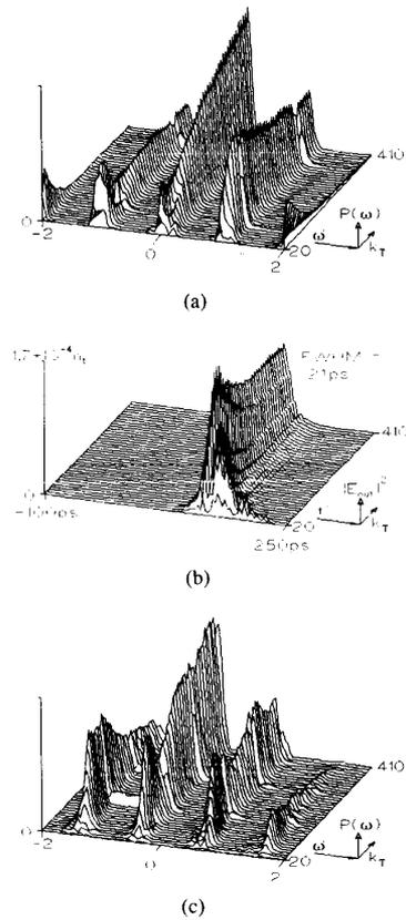
Fig. 10. Simulation of ring configuration with low feedback and low reflectivities (same parameters as in Fig. 9, but with  $R_{1,2} = 0.01$ ,  $J_{\text{max}} = 1.35 J_i = 2.8 J_{0.33}$ , where  $J_{0.33}$  is the injection current threshold for reflectivities of 0.33). (a) Power spectrum. (b) Temporal evolution of the output intensity. (c) Influence of the linewidth enhancement factor in mode-locking regime (same plot as in (a), but with  $\alpha = 3$  instead of  $\alpha = 0$ ).
