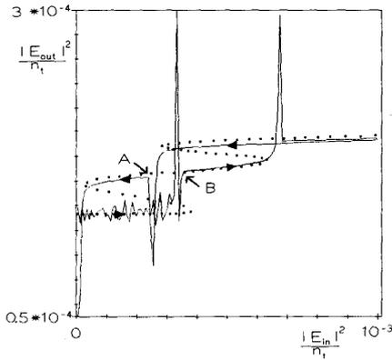
Fig. 5. Optical tristability, plotted as in Fig. 4, with  $J = 4J_r$ ,  $\omega'_{in} = -0.5$ ,  $\alpha = 7$ ,  $t_c = 16$  ns, and maximum  $|E_{in}|^2 = 10^{-3} n_t$ .
