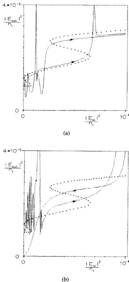
Fig. 4. Optical bistability: normalized optical output intensity is plotted versus optical input intensity for  $J = 1.2 J_t$  ( $J_t$ , threshold current density),  $\omega_{in}' = 0.25$ ,  $\alpha = 7$ , and (a)  $t_C = 33$  ns and (b)  $t_C = 4$  ns. (Full line: time-dependent numerical solution, dotted line: static analytical solution.)
