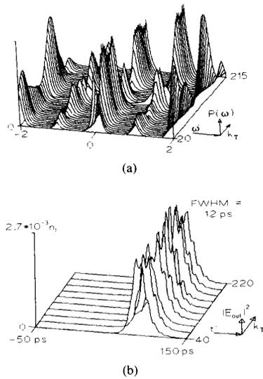
Fig. 8. Simulation of ring configuration with low feedback and high reflectivities (same parameters as in Fig. 7(a)–(c), but  $R_{\text{ext}} = 0.1$  and lower maximum injection current ( $J_{\text{max}} = 4.5 J_i$ ) in accordance with decreased effective dynamic threshold). (a) Power spectrum of output field. (b) Temporal evolution of output intensity.
