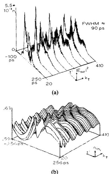
Fig. 13. Effect of too high an injection current ( $T_E = T_J = 512 \text{ ps}$ ,  $R_{1,2} = 0.01$ ,  $\alpha = 0$ ,  $R_{\text{ext}} = 0.5$ ,  $J_{\text{max}} = 1.3 J_i = 2.7 J_{0.33}$ ). The shortest pulses with FWHM = 20.8 ps were obtained for  $J_{\text{max}} = 0.8 J_i$ . (a) Temporal evolution of the output intensity. (b) Carrier density.
