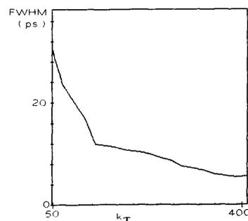
Fig. 12. Dynamics of pulse-compression: FWHM of output intensity is plotted versus index  $k_T$  that labels subsequent pulses, corresponding to number of round trips in ring configuration ( $\alpha = 0$ ,  $R_{\text{ext}} = 0.5$ ,  $J_{\text{max}} = 0.54 J_i = 2.8 J_{0.33}$ ,  $R_{1,2} = 10^{-5}$ ).
