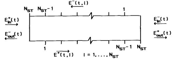
Fig. 1. Discretization scheme: traveling wave fields  $E^\pm(t, z)$  are replaced by  $E^\pm(t, i)$ ,  $i \in \mathbb{Z}$  with  $z = \frac{1}{2}[L \pm (-L + i2L/N_{\text{ST}})]$ ;  $L$  is length of SCLA, which is divided into  $N_{\text{ST}}$  equal intervals.
