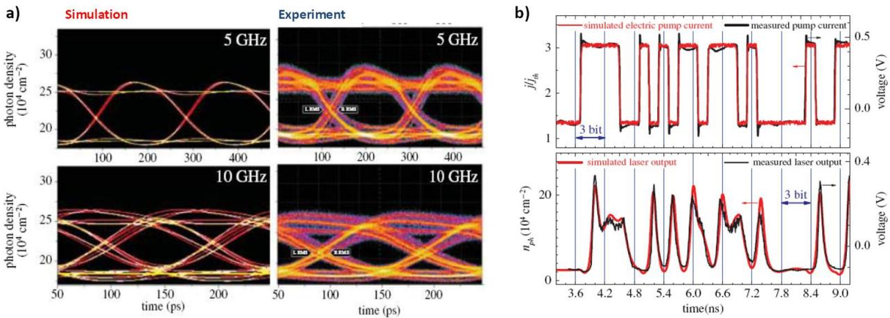
**Fig. 1:** (a) Simulated and measured eye pattern diagrams for pump currents switching between 4  $j_{th}$  and 6  $j_{th}$  ( $j_{th}$ : threshold current density) for bit repetition frequencies of 5 GHz and 10 GHz (b) Simulated (red line) and measured (black line) laser output (bottom) driven by an electric pump signal (top). After [P2].
