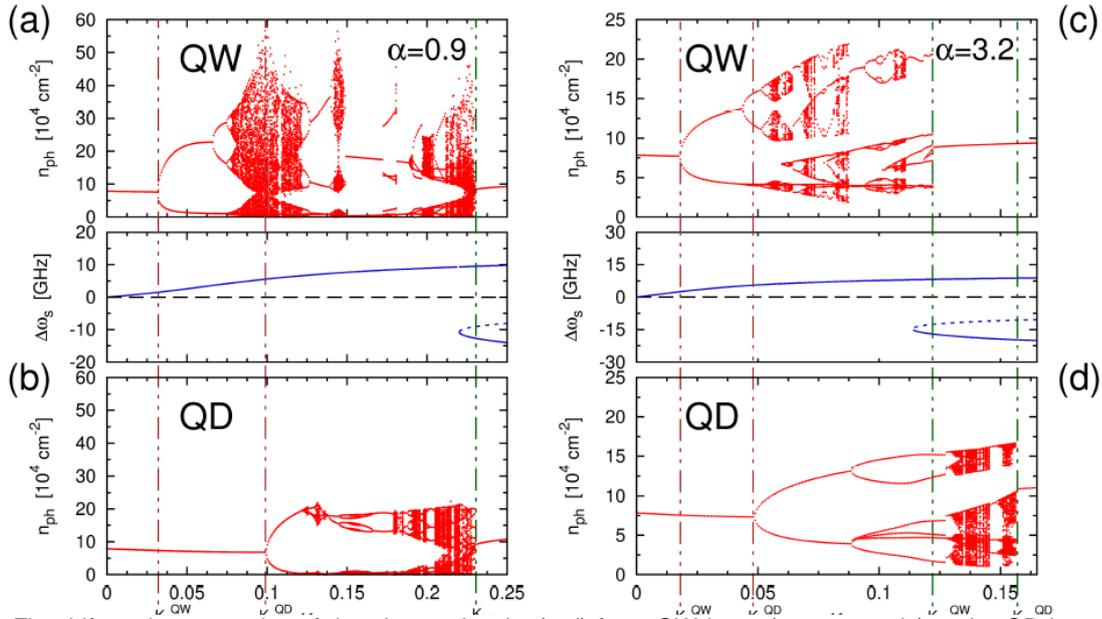
**Fig. 4:** First bifurcation cascades of the photon density (red) for a QW laser (upper panels) and a QD laser (lower panels) in dependence of the feedback strength  $K$  for  $\alpha=0.9$  ((a)-(b)) and  $\alpha=3.2$  ((c)-(d)). Middle panels: Frequency deviations of the possible external cavity modes (blue). Brown vertical dash-dotted lines mark the Hopf bifurcation. Green vertical dash-dotted lines mark the ends of the bifurcation cascades. After [P6].
