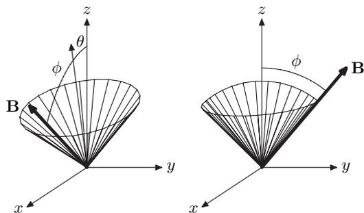
Fig. 4: Kinematics of the three-dimensional magnetic field. We simulate filaments actuated by magnetic fields that follow the surface of a cone with opening angle  $\phi$ , tilted at an angle  $\theta$  to surface normal (left) and a “hybrid” stroke (right) which consists of a rotation in the  $yz$ -plane as the propulsive stroke followed by a truncated cone with opening angle  $\phi$  oriented normal to the surface; both parts of the stroke are executed in equal time.
