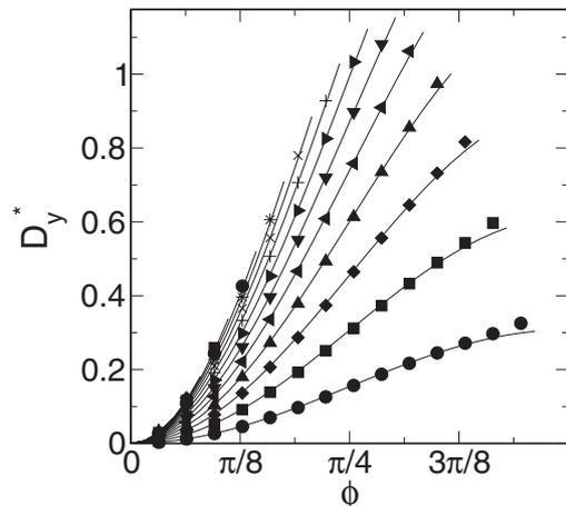
Fig. 5: Comparison between the theoretical prediction and the measured value of the pumping performance,  $D_y^*$ , for the tilted cone ( $Sp=2$ ). Each curve represents the results for different values of the opening angle,  $\theta$ , separated by  $\Delta\theta = 0.1$  starting from the bottom with  $\theta = 0.1$ . Measured values are given by points, the solid lines are a least-squares fit of the simulation data to  $C \sin^2(\phi) \sin(\theta)$ , where  $C$  is a constant.
