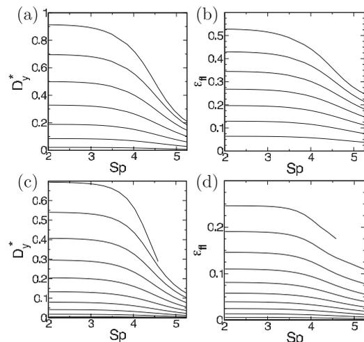
Fig. 6: Pumping performance  $D_y^*$  and  $\varepsilon_H$  as a function of  $Sp$ . (a, b) Tilted cone ( $\theta = \pi/4$ ): each curve corresponds to a different opening angle  $\phi$  with changes of  $\Delta\phi = 0.1$  (in radians) between curves up to a maximum  $\phi = 0.7$  (upper curve). (c, d) Hybrid stroke: each curve corresponds to a different opening angle  $\phi$  with spacing  $\Delta\phi = 0.1$  up to a maximum  $\phi = 1.1$  (upper curve).
