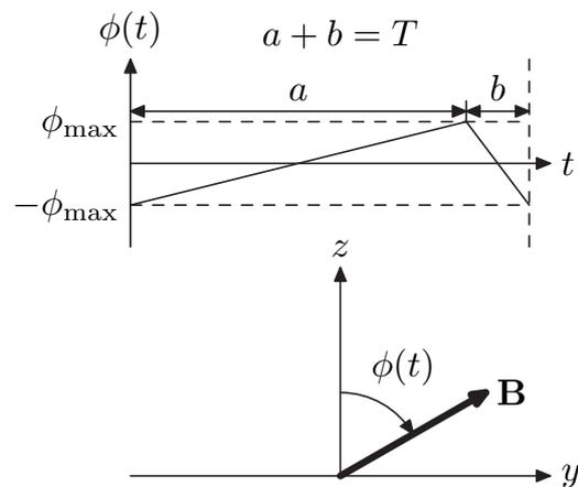
Fig. 1: Kinematics of the magnetic field: the field oscillates in the plane normal to the surface between the angles  $\pm\phi_{\text{max}}$ . Forward and backward strokes occur during time intervals  $a$  and  $b$ , respectively.
