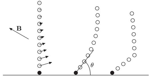
Fig. 3: Left: schematic showing the relative forces on beads in the lower half of the filament for a magnetic field at an angle to the filament. Middle and right: the relaxation of the filament in response to these forces for filaments with no defect and with a defect close to the surface. If a defect is present it can act as a lever which lowers the upper tip of the filament.
