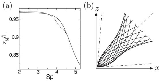
Fig. 7: (a) Maximum height of the filament tip for the tilted cone ( $\phi = 0.7$ , solid line) and hybrid ( $\phi = 1.1$ , dashed line) strokes. (b) Superimposed snapshots of a filament actuated by the tilted cone stroke ( $\phi = 0.7$ ,  $Sp = 5.3$ ). The dashed lines show the tilt axis and the upper and lower extents of the magnetic field.
