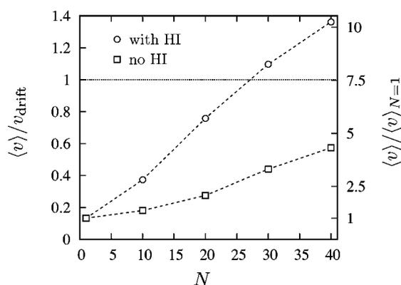
**Fig. 6** Mean velocity  $\langle v \rangle$  in units of  $v_{\text{drift}}$  (left ordinate) and  $\langle v \rangle_{N=1}$  (right ordinate) as a function of particle number  $N$ . The parameters are  $\omega_{\text{on}}t_{\text{diff}} = 4.5$ ,  $\omega_{\text{off}}t_{\text{drift}} = 3.6$ ,  $a = 0.1$ , and  $b = 100$ . The symbols refer to simulation results including ( $\circ$ ) and without ( $\square$ ) hydrodynamic interactions, respectively.
