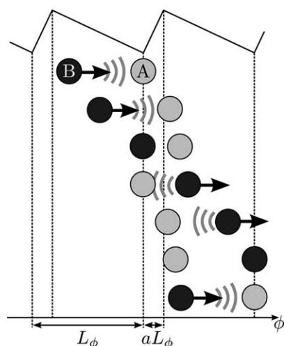
**Fig. 8** Transient cluster formation of a pair of particles using hydrodynamic interactions. The front and rear particles are labeled A and B, respectively. The colors of the particles indicate the on-state (black) and the off-state (grey) in the ratchet cycle. The arrows show the drift direction in the ratchet potential and the grey arcs symbolize hydrodynamic interactions between the particles. The picture is explained in detail in the main text.
