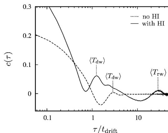
**Fig. 9** Velocity auto-correlation functions  $c(\tau)$  as a function of the rescaled time difference  $\tau/t_{drift}$ . Solid and dotted lines refer to data where hydrodynamic interactions (HI) are included or neglected, respectively. The mean periods  $\langle T_{dw} \rangle$  and  $\langle T_{rw} \rangle$  of the drift-wait and run-walk cycles are indicated in units of  $t_{drift}$ .
