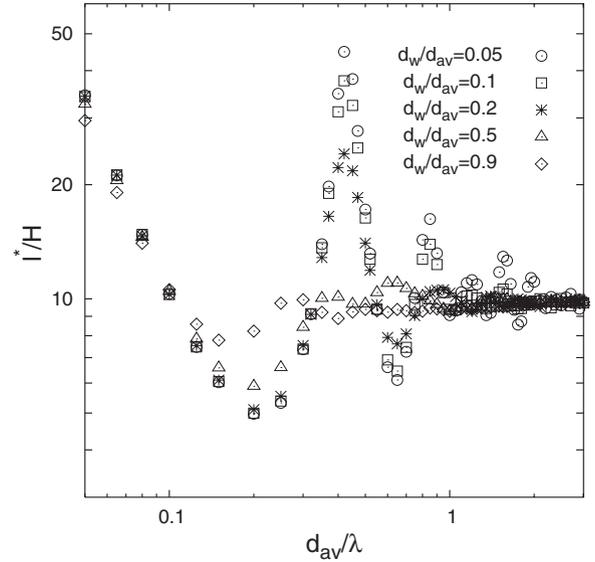
FIG. 8. The transport-mean-free path  $l^*$  (in units of the average cell diameter  $H$ ) as a function of  $d_{av}/\lambda$  for Voronoi foam 4 with various thickness distribution. Note, for  $d_w/d_{av}=0.5$  and  $0.9$ , the pronounced maximum disappears.
