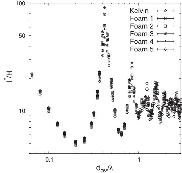
FIG. 6. The transport-mean-free path  $l^*$  (in units of the average cell diameter  $H$ ) as a function of  $d_{av}/\lambda$  for the Kelvin foam and disordered Voronoi foams 1–5. The refractive index  $n_0$  of the liquid phase is 1.34.
