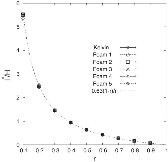
FIG. 4. The transport-mean-free path  $l^*$  (in units of the average cell diameter  $H$ ) as a function of intensity reflectance  $r$ , for the Kelvin and the disordered Voronoi foams 1–5. The Monte Carlo simulation results and the fit  $l^*(r)/H=0.63(1-r)/r$  are denoted, respectively, by points and line.
