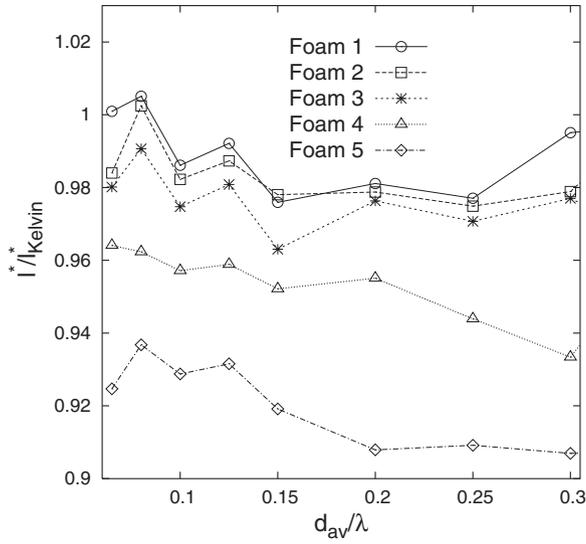
FIG. 7. The transport-mean-free path  $l^*$  of Voronoi foams 1–5 plotted relative to  $l^*_{\text{Kelvin}}$  as a function of  $d_{av}/\lambda$ . For all these foams,  $d_w=0$ .
