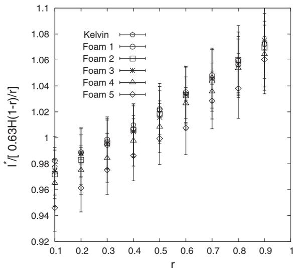
FIG. 5. The transport-mean-free path  $l^*$  plotted relative to  $0.63H(1-r)/r$  as a function of intensity reflectance  $r$ . We find that  $l^*_{Voronoi}(r)=0.63H(1-r)/r(1-b_1+b_2r)$  with  $0 < b_1 < 0.1$  and  $b_2 \approx 0.1$ .
